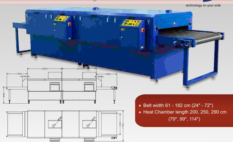
DEL series electric dryer is affordable multitask tunnel dryer. With its segmental chamber design provides choice of productivity capacities. The choice of belt widths (24" - 72") determines the max. curing element size. Compact transportation package foot print lowers transport cost and provides easy floor access.
